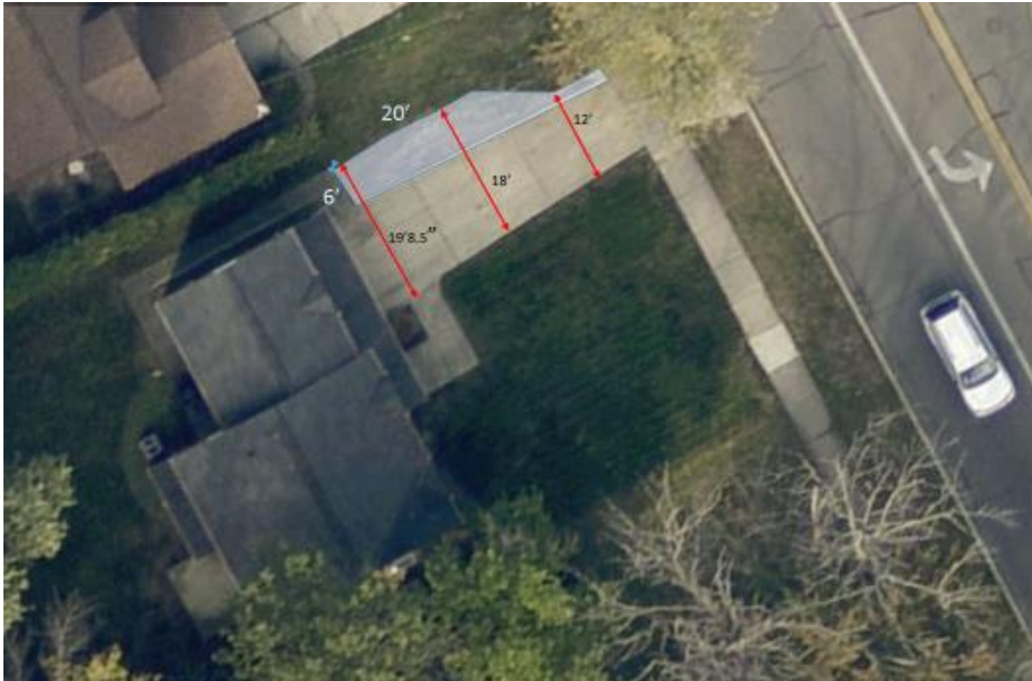
Proposed driveway parking area width from 19'8.5" to 17'3" and then narrows to the code conforming 12'. New pavement is 4'2" from the side property line
