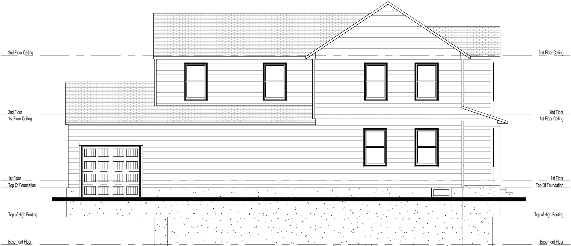
2 Left Elevation - Elev A 1/8" = 1'-0"
