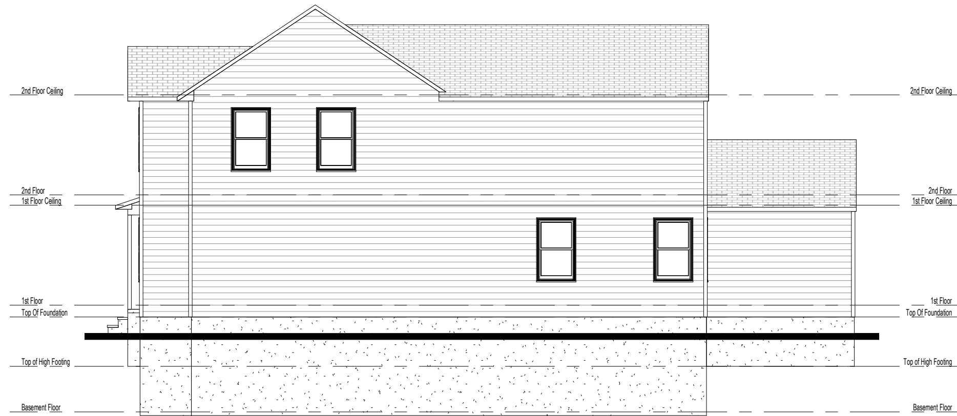
1 Right Elevation - Elev A 1/8" = 1'-0"
